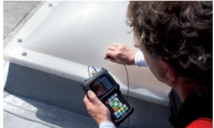
If necessary, a **non-destructive** before/after ultrasound measurement can be carried out to determine the layer thickness of KEMPEROL® FALLSTOP **once it is fully cured**. The ultrasonic thickness gauge is used to measure the correct layer thickness of between 0.7 and 0.9 mm.
