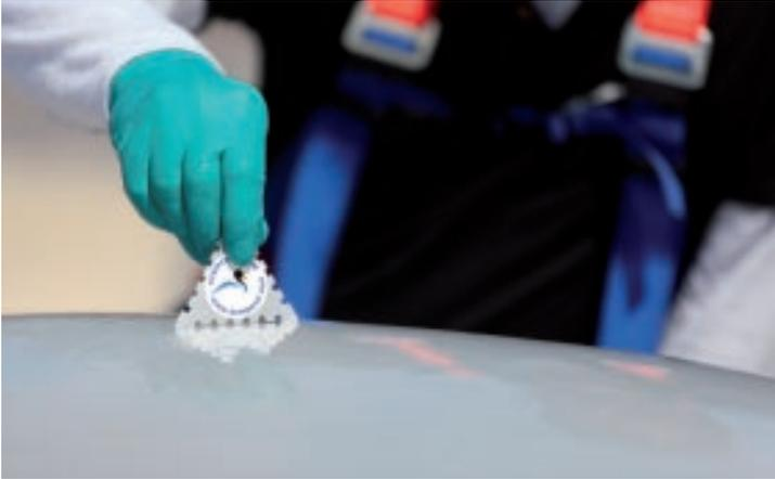
Note: At the end of each work step, the applied material is gauged at various points using the **KEMPERTEC® V4A measuring comb** (400 g/m<sup>2</sup> correspond to 400 µm).
